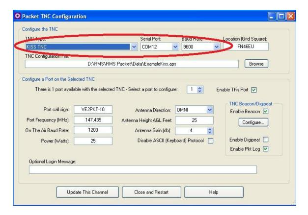
The Baud Rate MUST matches the one used in XRouter on the Interface use for the RMS.
