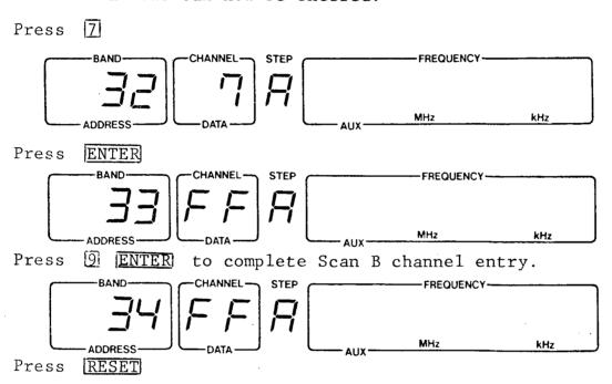
The A74 type microcomputer will ignore any entries made after pressing [SCAN] [B].
