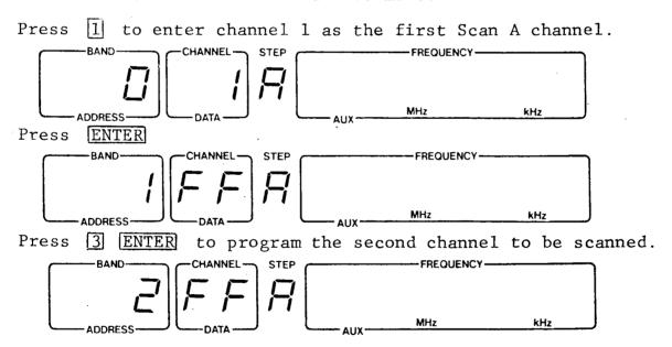
Scan A entries are now complete. To prepare for Scan B entries, press  $\boxed{\square}$  and hold until the BAND/ADDRESS display shows 32.
