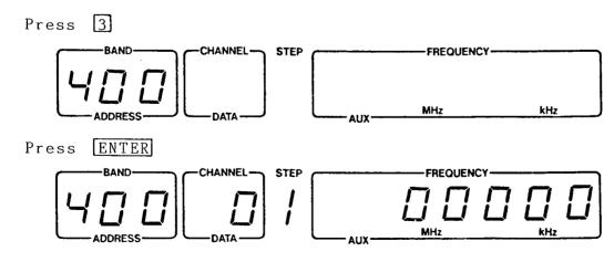
A BAND display of 400 is indicated and the 70--1000 is ready for channel programming.
