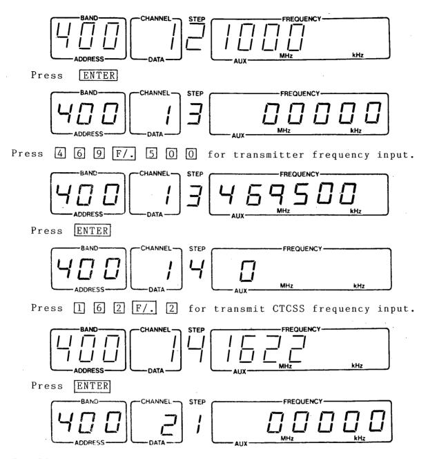
The 70-1000 is now ready for the Receiver and Transmitter information to be entered for channel "2".
